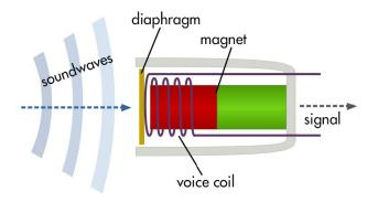
The **dynamic microphone** is an electroacoustic transducer, that transforms sound pressure pulses (according to the principle of electromagnetic induction) into electrical voltage pulses.
